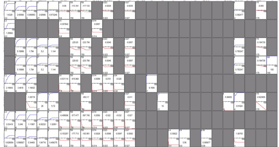
Example of a moderately-sized gain matrix from the Burnaby Refinery.
